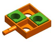
Figure 2.5: Assembly-aid-tray for bearing boxes
