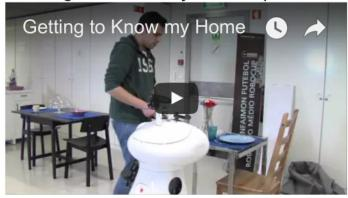
The robot is supposed to generate a semantic map of the apartment. How this is achieved is not specified, for example a team can guide the robot through the apartment, or the robot can explore it fully autonomously.
