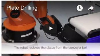
In this task the robot has to pick up a cover plate from a conveyor belt, conduct a quality check and perform one of three tasks according to the quality of the plate: perfect - collect; unusable - throw
