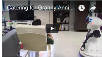
In this task the robot has to manage different day to day tasks. Granny Annie can call for the robot via her tablet computer. On arrival it can be given commands to, for example lift the shutters, tilt the window and switch of the lights. Another task may be to search for and bring back her reading glasses.
