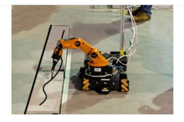
The robot has to follow a straight line/spline (without sensor feedback). Using a marker mounted on its end-effector an external system measures the path accuracy.
