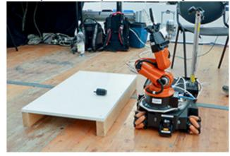
The robot has to identify the object in front of it, grasp and lift it and release it after a given time. The pose of the object in the gripper is not important, as long as the object is succesfully grasped.
