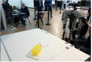
From a set of objects the robot has to detect, recognize and locate an object placed in front of it. Objects could be for example a tray, an axis or a bearing box.
