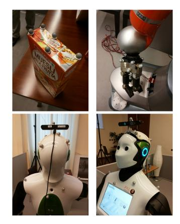
Figure 3.1: Examples of installation of markers (gray spheres) at the 2014 RoCKIn Camp. Clockwise from top left: on a box (the box had to be grasped by robots); on the wrist of a robot; on the back and front of the head and torso of a robot.
