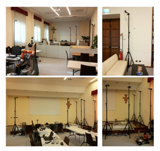
Figure 3.3: Motion capture cameras as installed at the 2014 RoCKIn Camp. On the left, camera setup around the RoCKIn@Home (up) and RoCKIn@Work (down) testbed. On the right, closer views of a single RoCKIn@Home tripod with camera (up) and of part of the RoCKIn@Work setup (down).
