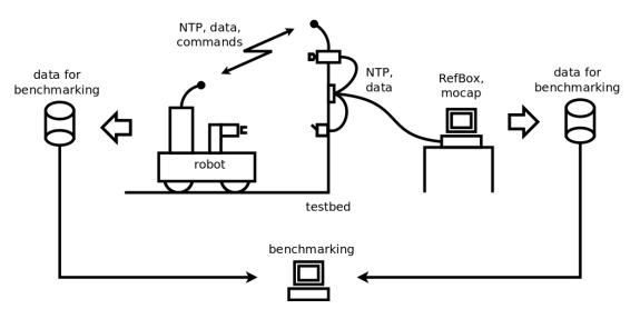
Figure 2.2: Simplified view of the architecture of the RoCKIn data collection and processing system for benchmarking.
