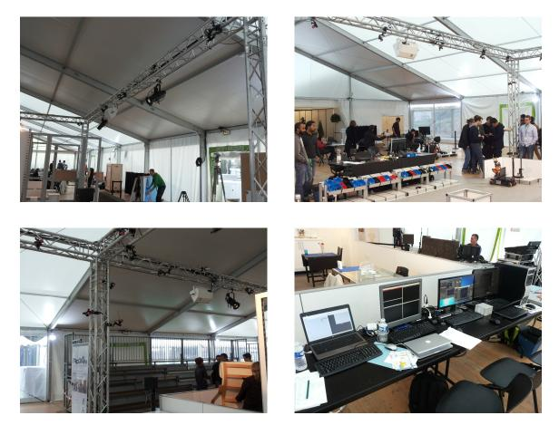
Figure 4.3: Four snapshots of the benchmarking system at Toulouse. Clockwise from top left: trusswork with cameras (and spotlights) above the RoCKIn@Home testbed; trusswork above the RoCKIn@Work testbed; some of the PCs used by the Benchmarking System; motion capture cameras used for FBM1.
