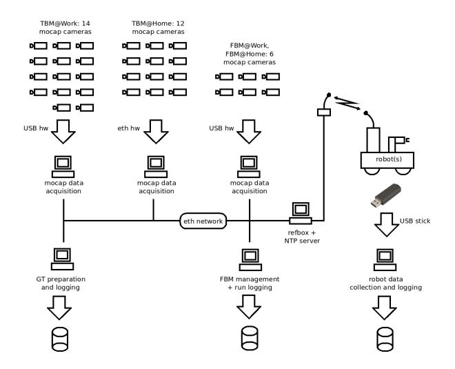
tle PC #2). Each system has a Windows PC to run the Optitrack Motive software <sup>1</sup>, which is required to interface with the cameras and track the marker sets. Processed data is streamed over UDP to the clients.
