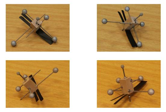
Figure 4.4: Four different views of one of the marker sets used at the 2014 RoCKIn Competition.
