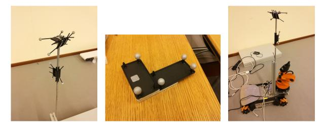
Figure 3.4: Two examples of rigid bodies fitted with markers, and a robot equipped with one of them.
