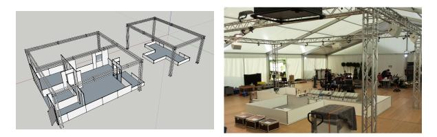
Figure 2.1: Left: CAD sketch of the testbeds, showing the trusses dedicated to supporting the motion capture cameras. Right: the actual truss built above the RoCKIn@Work testbed at the 2014 RoCKIn Competition in Toulouse. The little black objects underneath the truss are motion capture cameras on adjustable mountings.
