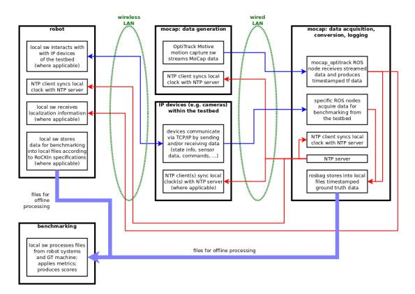
Figure 2.3: Architecture of the RoCKIn data collection and processing system for benchmarking. The modules in this Figure are the same of Figure 2.2.
