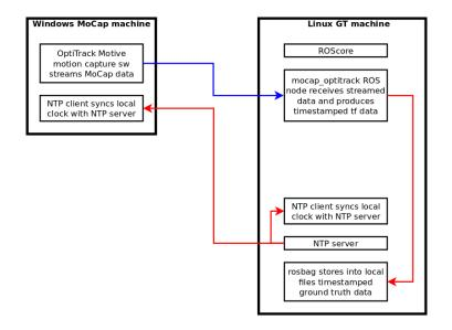
Figure 3.2: System used at the 2014 RoCKIn Camp to acquire and log trajectory data from the motion capture system. This is a subset of the system shown in Figure 2.3.
